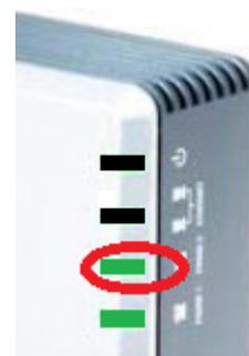
6/ Connect the Ethernet port of your computer to the socket "ETHERNET" of your IBRANTA box using another Ethernet cable (Check that your computer's network card is in DHCP mode so that the IBRANTA box automatically assigns you an IP address).
